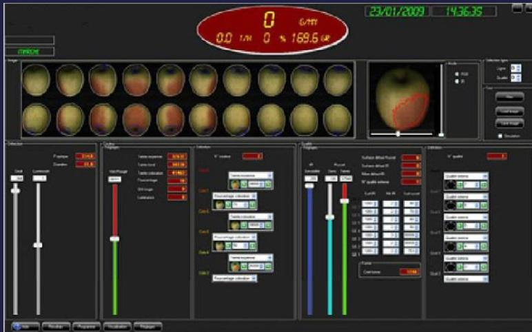
**Figure 1:** A 3D display provides the operator with information on a piece of fruit's size, colour, and any defects.
