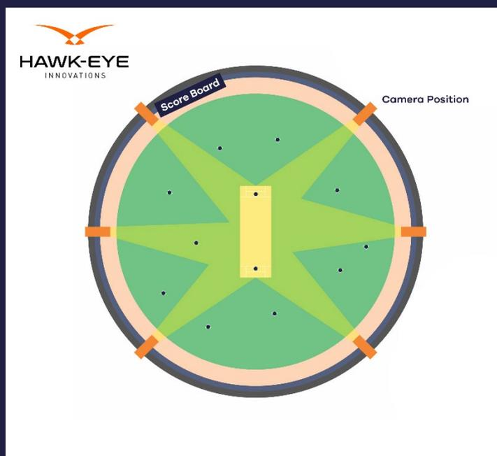
The six cameras are gen-locked into two sets of three cameras, each set being captured by a Matrox frame grabber and the Matrox Imaging Library (MIL-Lite) software. The resulting images are processed into a 3D image by the Hawk-Eye system which then calculates - in a split second - where the ball pitched, the extent of its lateral movement in the air and off the wicket, its
