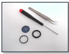
Screwdriver or Tweezers are recommended to remove retaining ring, but **are not included**. Retaining Ring will turn Clockwise to install and Counter-Clockwise to remove. There are 2 small holes and 2 slots in ring to install/remove.
