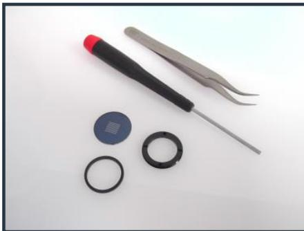
Screwdriver or Tweezers are recommended to remove retaining ring, but **are not included**. Retaining Ring will turn Clockwise to install and Counter-Clockwise to remove. There are 2 small holes and 2 slots in ring to install/remove.
