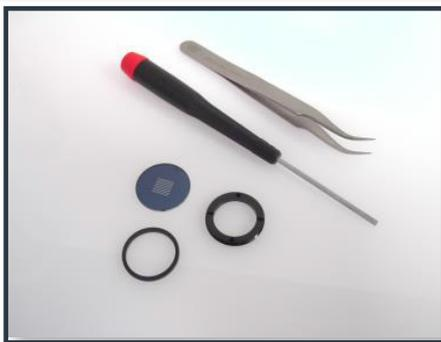
Screwdriver or Tweezers are recommended to remove retaining ring, but **are not included**. Retaining Ring will turn Clockwise to install and Counter-Clockwise to remove. There are 2 small holes and 2 slots in ring to install/remove. Install the skinny metal side of pattern towards the LED
