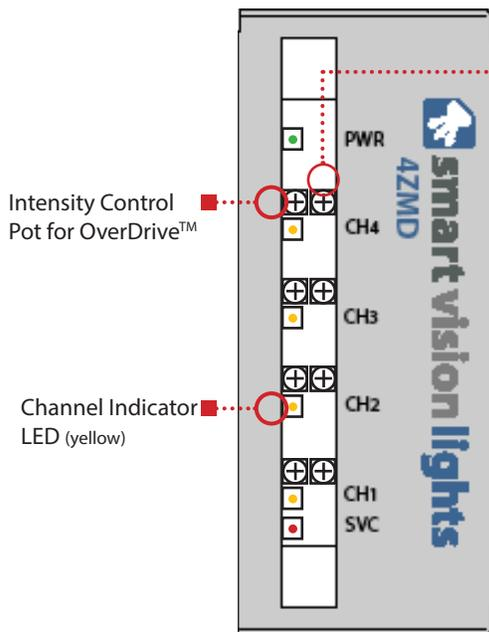
Intensity Control Pot for Continuous Operation
