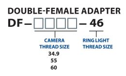
\*When mounting an EZ Mount Ring Light, a double-female adapter is used.
