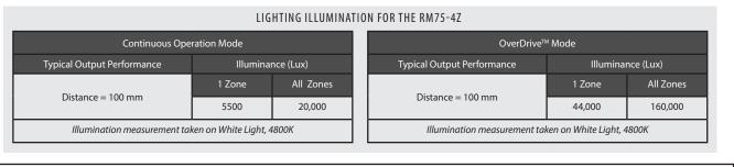
Smart Vision Lights recommends using the RM75-4Z be used at a working distance between 50 mm and 200 mm.
