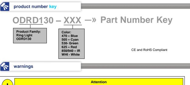
Attention Please note that the power requirements are up to 4A at 24VDC. Failure to supply light with up to 4A can result in non-repeatable lighting.
