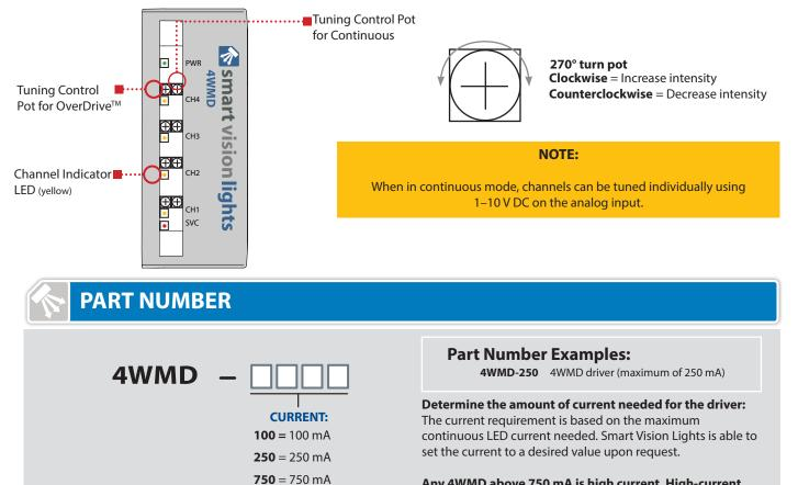
Any 4WMD above 750 mA is high current. High-current version is equipped with a cooling fan. 4WMD-2000 is the high current version.
